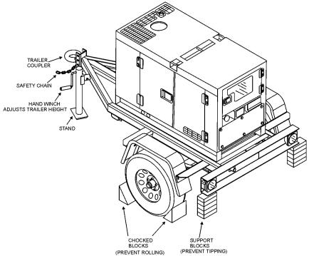
Figure 1. DCA-15SPX3 and Towing Trailer
